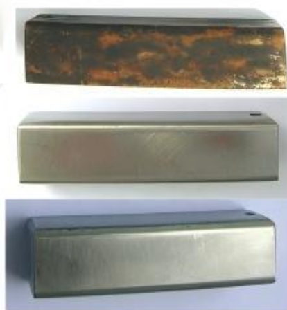
Figure 2. The macroscopic morphologies of A3 (Q235) steels after immersion in ethylene glycol, ET-1 and ET-4 solutions for 168 hours is shown from top to bottom
