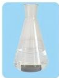
Figure 3 50% Ethylene glycol The solution is become turbid, and 90% of the carbon steel test piece is corroded
