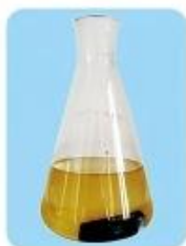
Figure 1 Water The water is turbid, and the carbon steel test piece is corroded
