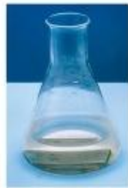
Figure 5 50% Ethylene glycol The carbon steel test piece is severely corroded, and the rust accumulates and deposits on the bottom
