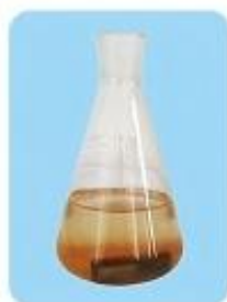
Figure 1 Water The water is turbid, and the carbon steel test piece is corroded
