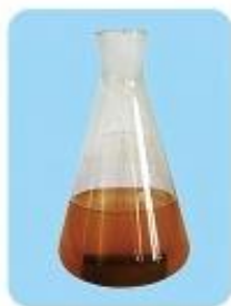
Figure 3 50% Ethylene glycol The solution is become turbid, and 90% of the carbon steel test piece is corroded
